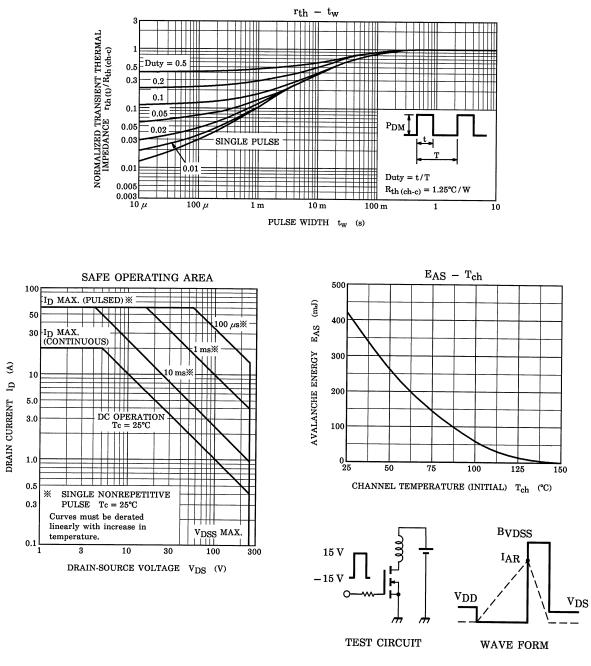
$$\begin{array}{l} \mathrm{R_{G}=25~\Omega} \\ \mathrm{V_{DD}=90~V,~L=1.79~mH} \end{array} \qquad \mathrm{E_{AS}=\frac{1}{2}\cdot L\cdot I^{2}\cdot \left(\frac{\mathrm{B}\mathrm{VDSS}}{\mathrm{B}\mathrm{VDSS}-\mathrm{VDD}}\right) } \end{array}$$
